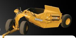
The dolly-wheeled scraper features the same quality as our direct-mount style, but with no need for a specialized scraper drawbar. Perfect for agricultural and industrial use, the weight of this scraper and its payload are carried entirely by front and rear wheels. The front dolly wheels also provide excellent ground following ability, independent from your tractor. If you do not have full-time scraper work, the dolly-wheeled style will allow you the freedom to easily switch between power units.
